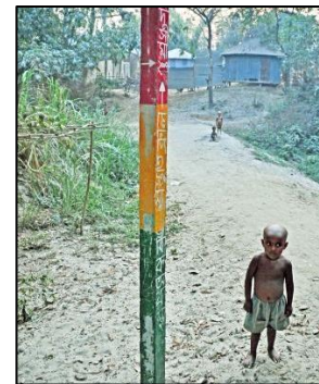
A flood meter measures water levels during the monsoon in Bangladesh. Photo by Robert Friedman, USAID.
