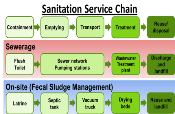
Figure 2: Effective and sustainable sanitation requires an approach that considers the entire continuum of sanitation services, from initial containment through final reuse and/or disposal, referred to as the sanitation service chain.
