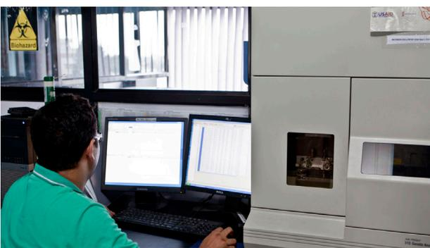
The Applied Biosystems' (USA) ABI 310 Genetic Analyzer was acquired through the NTGP as part of enhancing the laboratory capacity of CMDN to perform comprehensive genetic analysis of tiger scat samples. It allows NTGP team to identify individual tigers from scat DNA.
