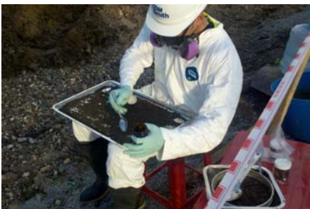
Confirmation soil sampling (Photos: CDM Smith)
