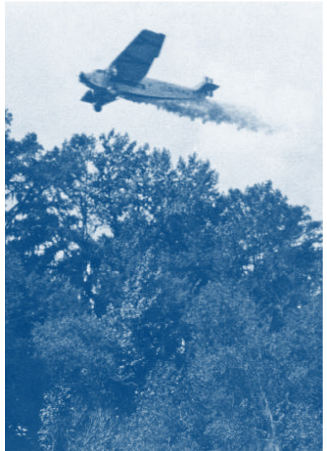
A Ford Trimotor sprays insecticide in the southern United States to control malaria-carrying mosquitoes. Credit: CDC
