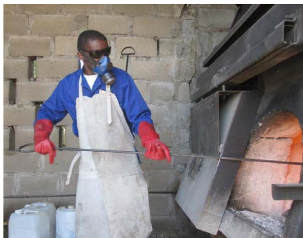
Proper PPE is crucial for individuals handling waste and operating incinerators to reduce associated risks, including physical injury or inhalation of exhaust.
